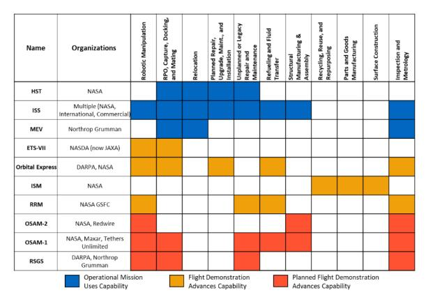
Figure 2: Operational missions and flight demonstrations have used and advanced ISAM capabilities, and planned missions will demonstrate more. Robotic Manipulation; RPO, Capture, Docking, and Mating; and Inspection and Metrology capability areas have been used in most of these missions, and the ISS has used and demonstrated many of these ISAM capability areas.
